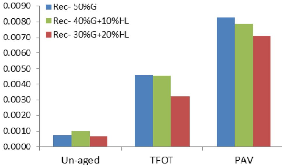
On an infrared spectrum, carbonyl groups formed by oxidative ageing (C=O groups) appear at around wavenumber  $1700\text{cm}^{-1}$ . The Carbonyl Ageing Index is the ratio of the carbonyl infrared response to the total infrared response. Fewer carbonyl groups are formed on ageing in mastics containing hydrated lime. Ageing was conducted by Thin Film Oven Testing (TFOT) or Pressure Ageing Vessel (PAV).
