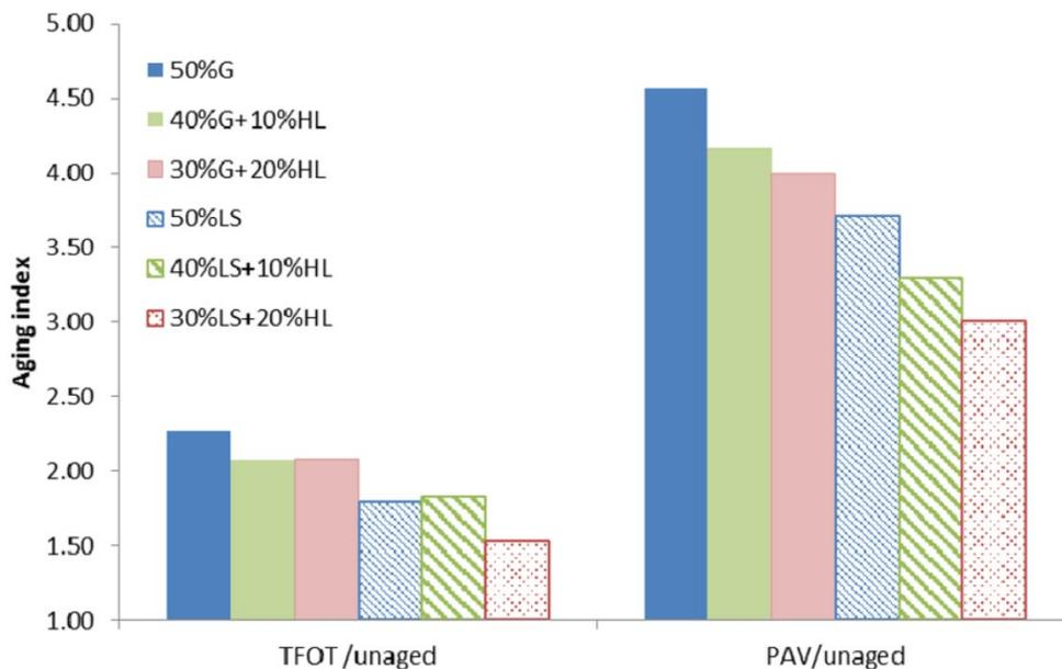
$G^*$  is the complex shear modulus for the mastic specimens and the  $G^*$  Ageing Index is the ratio of  $G^*$  (aged) over  $G^*$  (unaged). No change in  $G^*$  would have an Ageing Index = 1. The closer the Ageing Index is to 1, the smaller the change in  $G^*$  experienced upon ageing.
